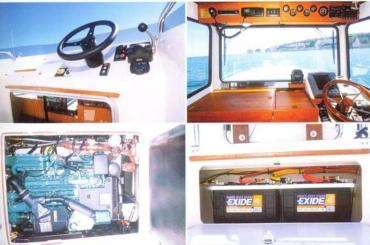
7.97 m L.o.a. Length (hull) 7.46 m 2,80 m Beam 0,80 m Draught Weight approx. 3100 kg Fuel tank 340 L 147-231 kW Engine (200-315 HP) 30 - 37 K.T. Speed Cruising speed (230 HP) approx. 28 K.T. Fuel consumption (230 HP) approx. I,6 L/N.M.
